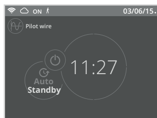
Pilot wire = Stop (Heating standby mode)
